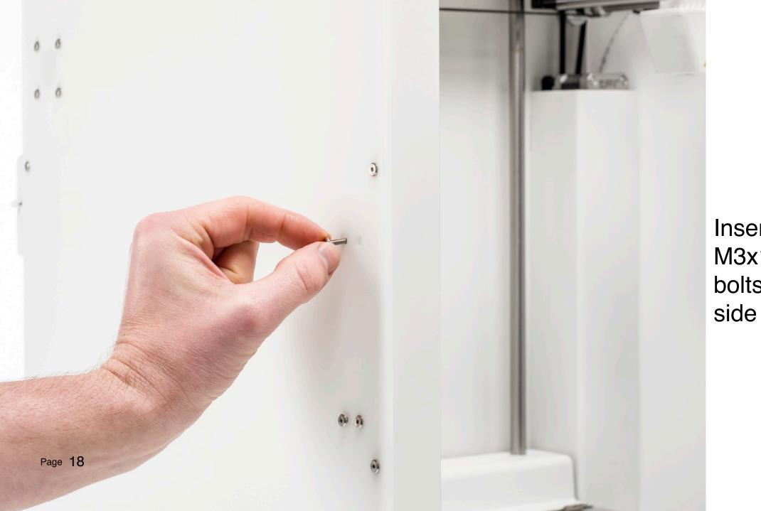
Insert the four M3x12 flathead bolts through the side panel
