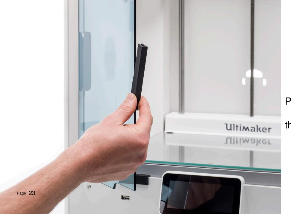
Place the alignment tool middle onto the glass door
