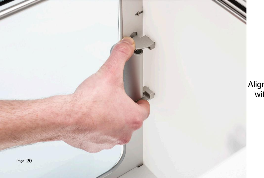
Align the hinge with the bolts
