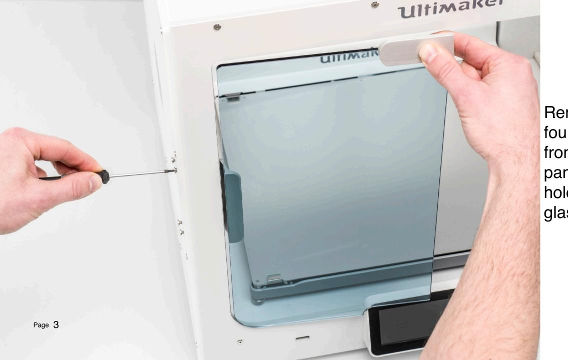
Remove the four bolts from the side panel, while holding the glass door
